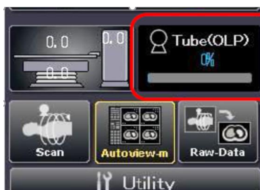
Figure 1. 21. Tube warm-up a warm-up was performed as OLP showed zero.
