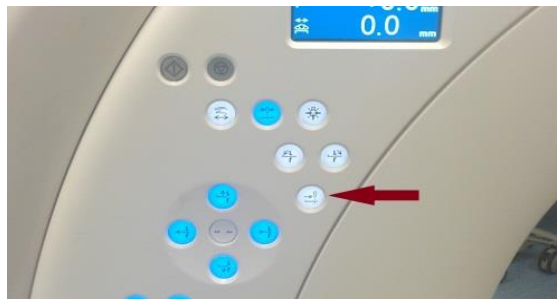
Figure 1. 25. Arrow showing phantom is centred using the zero button on the panel.
